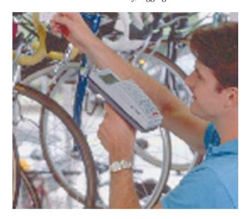
When alphanumeric input is required, the 35 - or 46-key sealed rubber keyboard enables simple and accurate manual keying. A supertwist LCD backlit display features large characters for easy reading. And, the 16-bit DOS architecture provides easy development of demanding interactive programs for retail and industrial applications.
